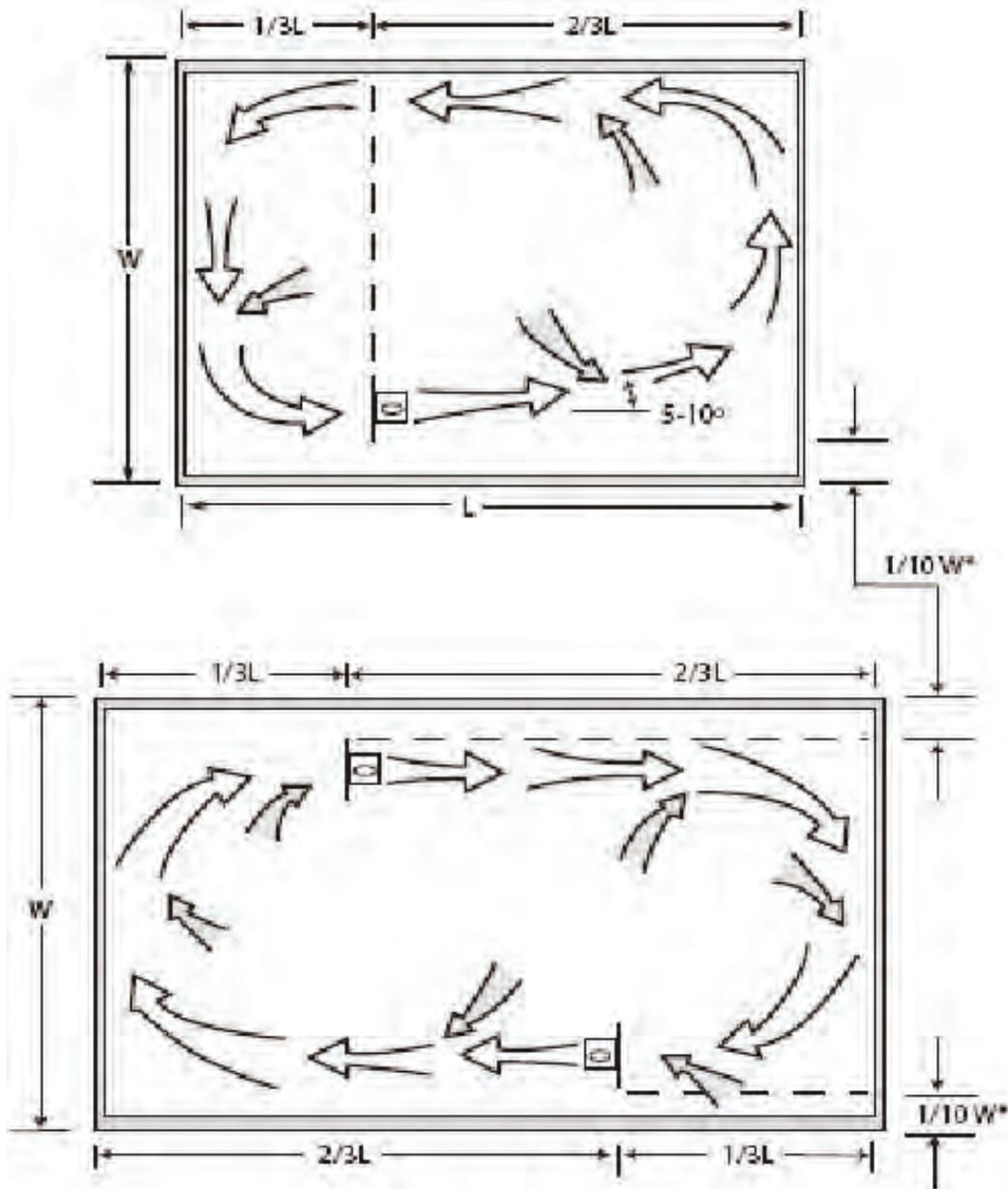
\*Inlet flange edges should not be more than 5 ft. from wall, regardless of shop width ( $W$ ).
