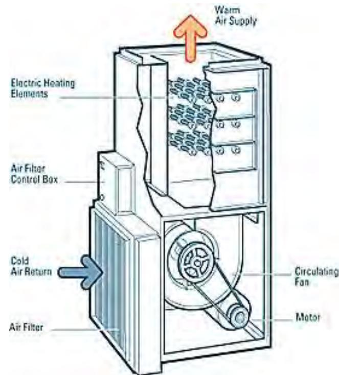
**Improve Filter Efficiency in Heating, Ventilating, and Air Conditioning System**
