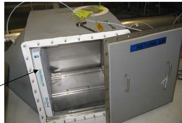
Modified in-duct air cleaner test loop with bypass
