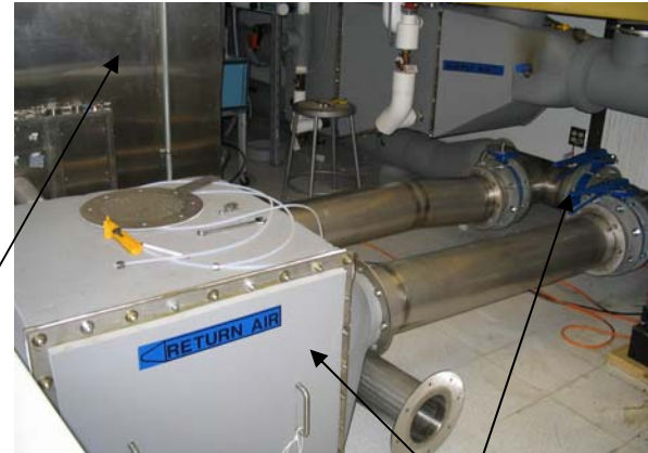
Modified in-duct air cleaner test loop with bypass
